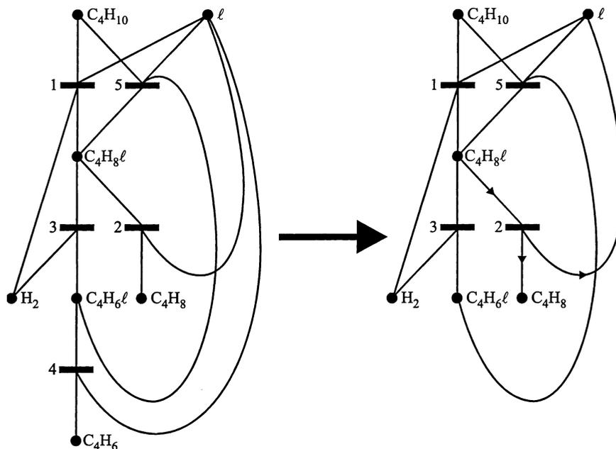
Fig. 3. Reduction part of algorithm RPIMSG for the dehydrogenation of butane to butene.
