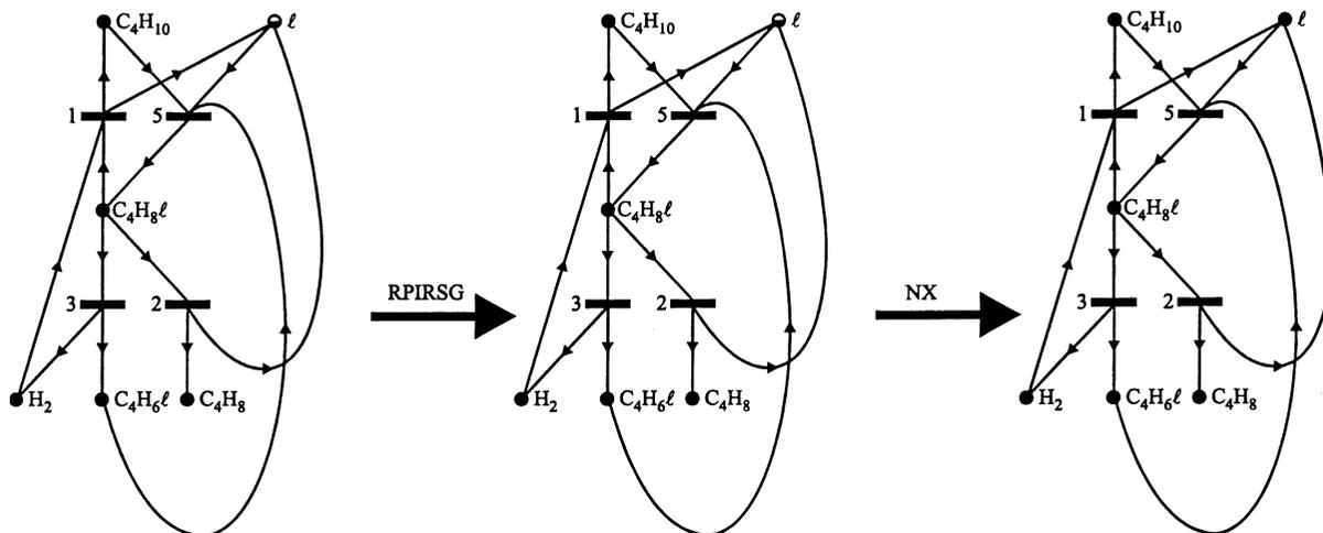
Fig. B.13. Step 6 resulting in combinatorially feasible structure 3.
