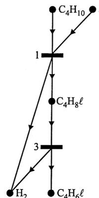
Fig. 1. P-graph representation of the network comprising elementary-reaction steps  $1 \rightarrow$  and  $3 \rightarrow$  in the pathway of the dehydrogenation of butane to butene.
