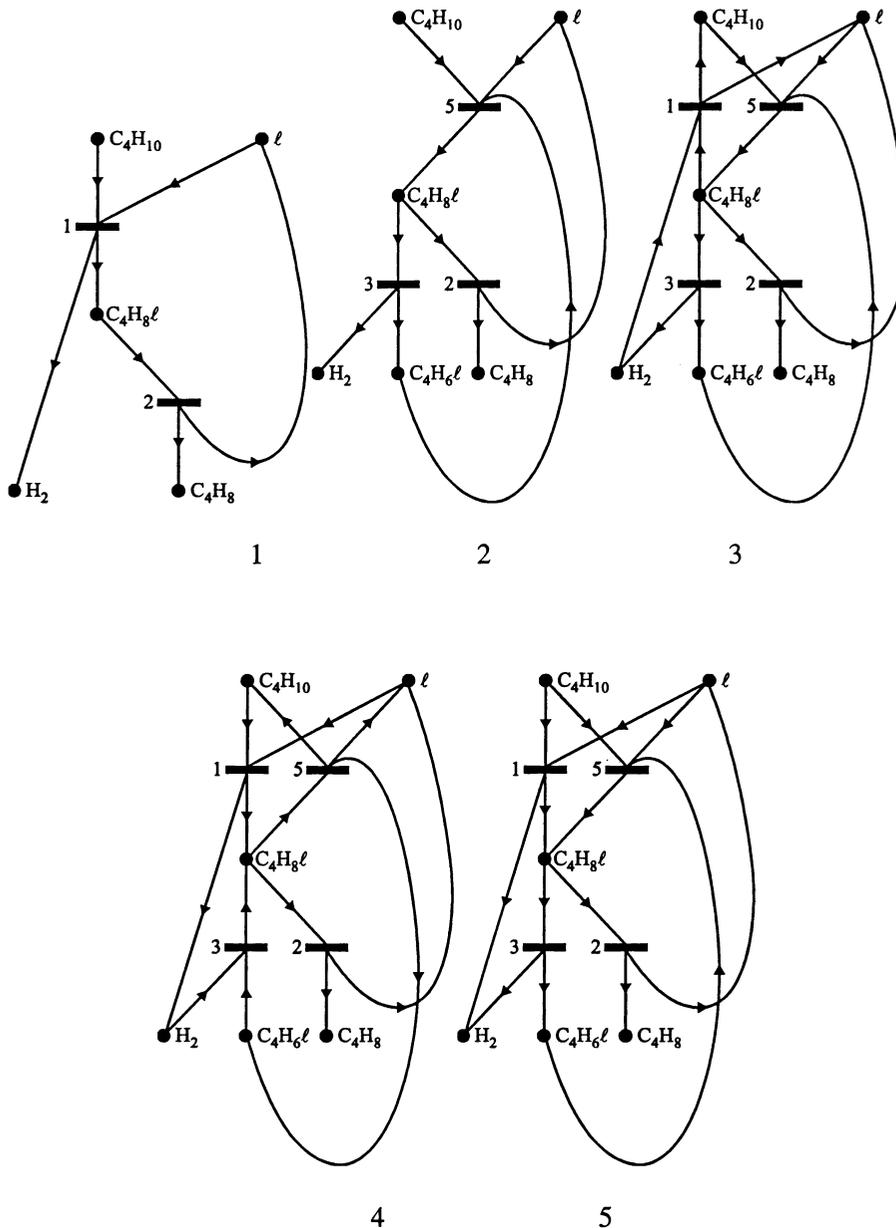
Fig. 7. Combinatorially feasible reaction networks for the dehydrogenation of butane to butene.
