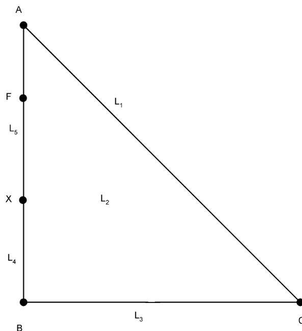
**Figure 6.** Simple system illustrating the identification of separators for eluding the thermodynamic pinches: A and B, desired products; F, feed; X, binary azeotrope of A and B;  $L_1$ , lumped material occupying line AC;  $L_2$ , lumped material occupying area ABC;  $L_3$ , lumped material occupying line BC;  $L_4$ , lumped material occupying line AX;  $L_5$ , lumped material occupying line XB.
