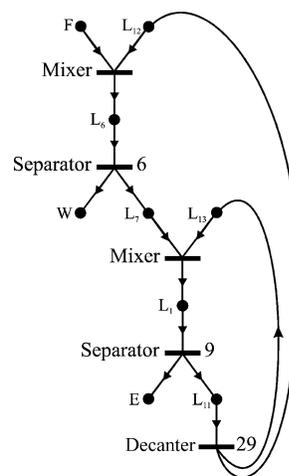
**Figure 8.** Structures 2684 and 2721, which are feasible and optimal, represented by a P-graph.
