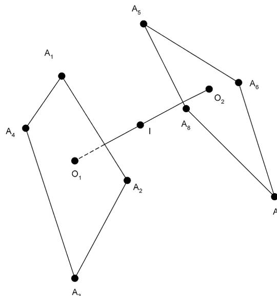
**Figure 5.** Representation of a decanter in the RCM with input I and outputs  $O_1$  and  $O_2$ , which are on the bounding planes,  $A_1A_2A_3A_4$  and  $A_5A_6A_7A_8$ , of the corresponding liquid–liquid equilibrium envelope, respectively.
