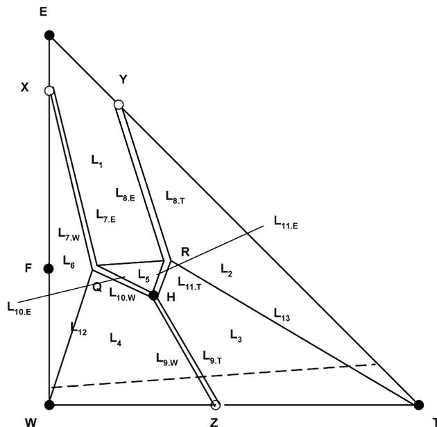
**Figure 2.** Linearized RCM of the ethanol (E)–water (W)–toluene (T) system illustrating the partitioned materials.
