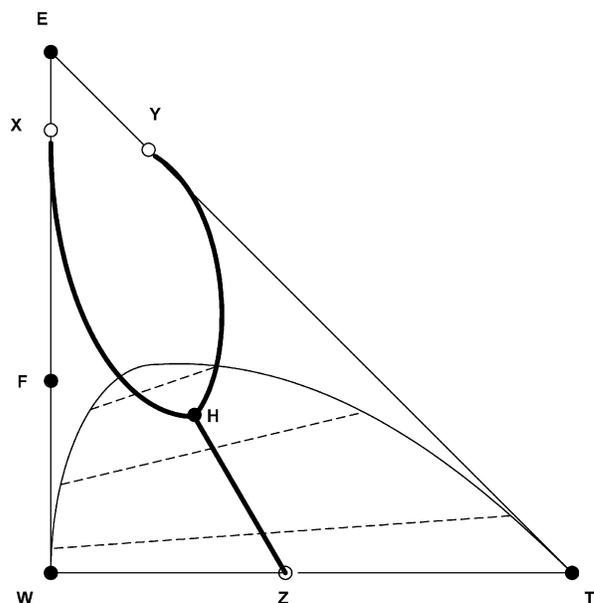
**Figure 1.** RCM of the ethanol (E)–water (W)–toluene (T) system: F, feed; X, Y, Z, binary azeotropes; H, ternary azeotrope.
